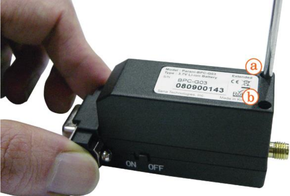
Figure 2-7 Fasten the battery pack
