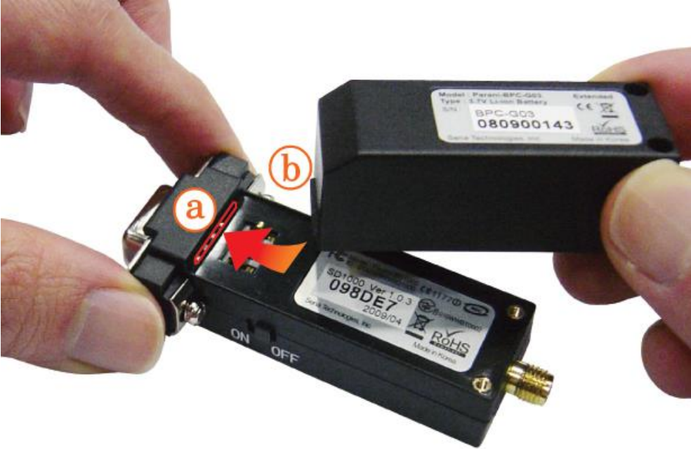
Figure 2-6 Attach the battery pack
