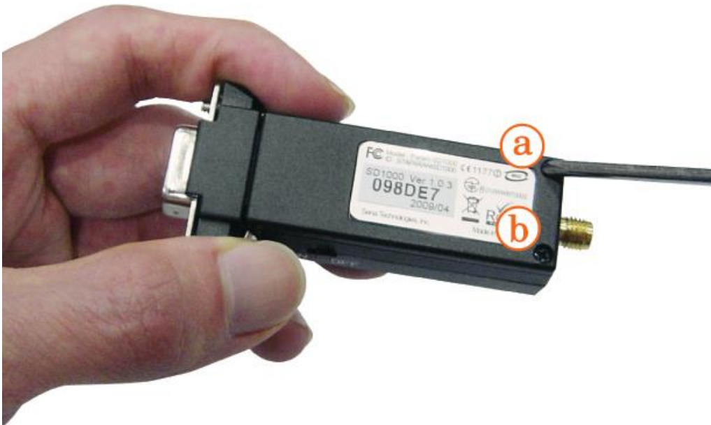
Figure 2-5 Remove Parani-SD1000 bottom cover
